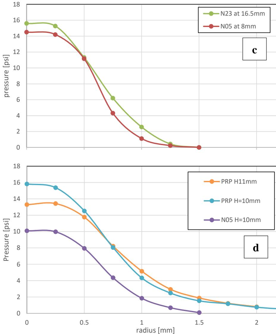
**Fig. 2:** Single jet nozzle pressure comparisons: a) Reference case – single 0.5mm jet and its dependence on distance from the impinged surface; b) comparison of wet (saline droplets) vs. dry working conditions; c) comparison to a wider single jet – 0.8mm, which requires greater working distance; d) comparison to the same diameter jet with the addition of an air shield – generates a wider impinged zone.
