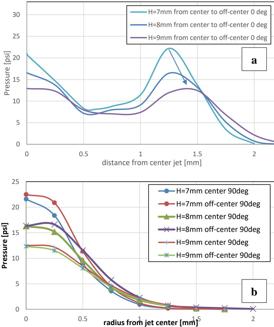
**Fig. 3:** Multi jet nozzle pressure comparisons: a) Triple 0.5mm jets inline (0 degrees), pressure along this line and its dependence on distance from the impinged surface; b) comparison of
