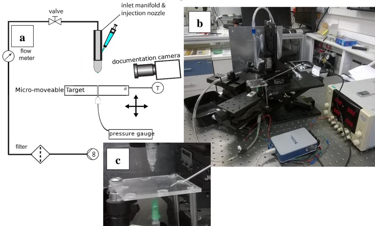
**Fig. 1:** Experimental system setup: I) schematic of layout; II) photo of system; III) close-up of nozzle, and micro-pressure measurement in the target (green needle)
