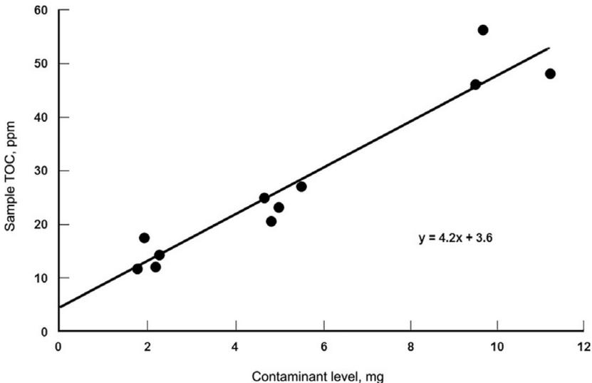
FIGURE 18.8 TOC vs the initial contaminant level of the stainless steel plates [22].
