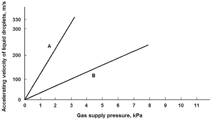
**FIGURE 18.10** Graph showing the relation between the velocity of the liquid drops and the supply pressure of the gas for different jet nozzles. A. Two-fluid nozzle. B. Conventional low-pressure nozzle [84].
