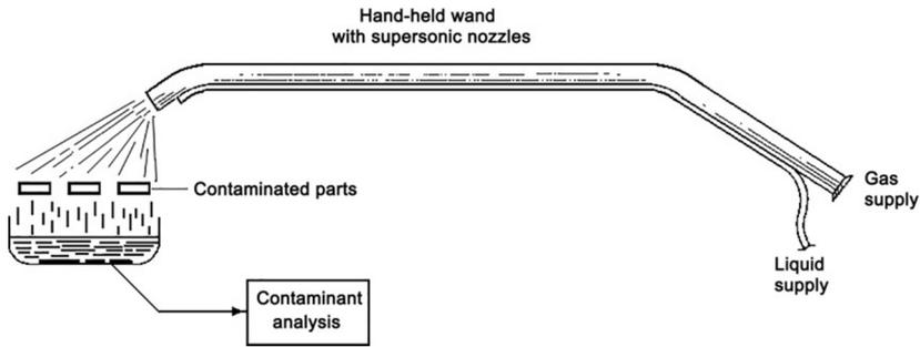
**FIGURE 18.4** Supersonic gas-liquid cleaning system arranged for precision cleaning and cleanliness verification [23].
