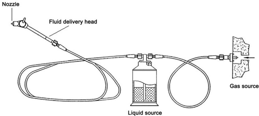
FIGURE 18.5 Schematic of the cleaning system for medical applications [57,61,62].
