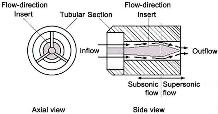
FIGURE 18.2 Converging-diverging nozzle with flow-directing annular insert [31–33,57].
