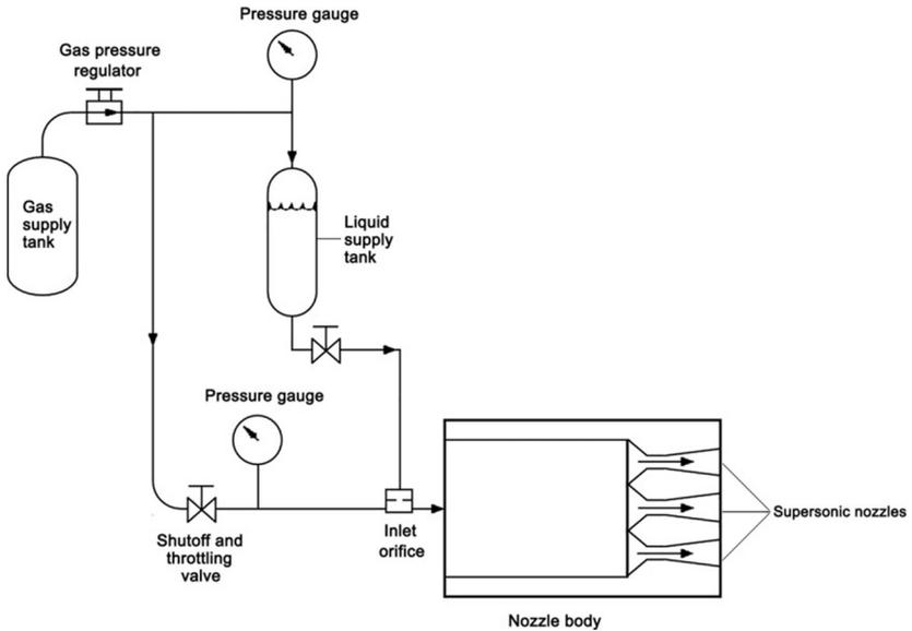
FIGURE 18.3 Schematic of the basic supersonic gas-liquid cleaning system for precision cleaning applications [22,23].
