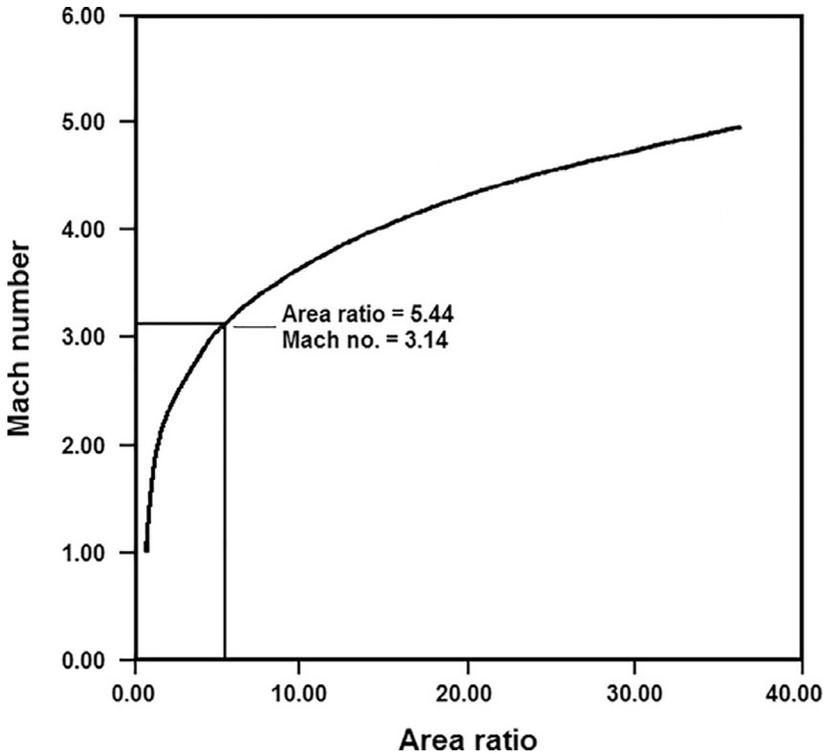
FIGURE 18.1 Mach number vs area ratio for the KSC SS-GLC converging-diverging nozzle [22].
