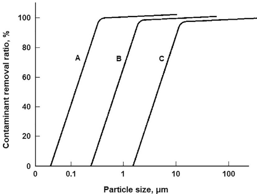
**FIGURE 18.11** Plot showing the relation between contaminant removal ratio and particle size with different jet cleaning nozzles. A. New two-fluid nozzle. B. A conventional low-pressure nozzle. C. A conventional high-pressure nozzle [84].
