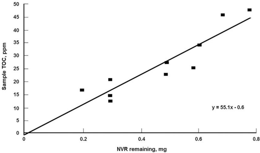
**FIGURE 18.9** Linear correlation between TOC and NVR remaining after cleaning [22].
